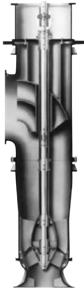
FIGURE 114 Vertical pull-out design allows the rotating element and critical non-rotating wear components to be removed for inspection and replacement without removing the complete pump (Flowserve Corporation)
