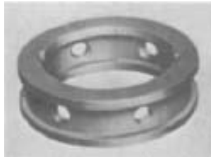
FIGURE 75 A lantern ring (also called a seal cage)
