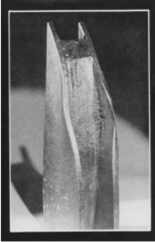
FIGURE 31 Damage to impeller from low-flow operation (Source: E. Makay in Power )
