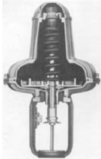
FIGURE 38 Diaphragm-and-spring actuator, reversible type (Foxboro)
