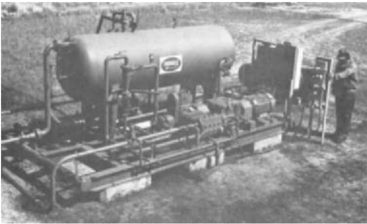
FIGURE 10 One-well unitized system (National Supply)
