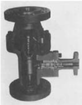
FIGURE 29 Pump bypass flow at high pressure drop results when line flow at top ceases and mechanism opens valve at right (Yarway).
