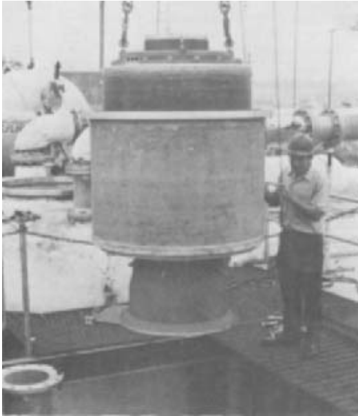
FIGURE 6 Ship-loading cryogenic pump (J.C. Carter Company, Inc.)
