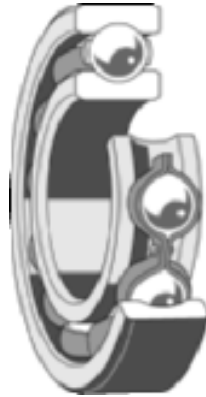
FIGURE 88 Single-row, deep-groove ball bearing (SKF USA, Inc.)
