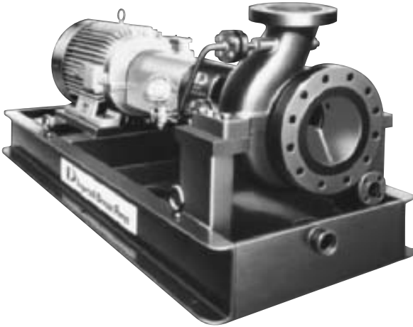
FIGURE 98 Horizontal shaft overhung pump and driver on a structural steel bedplate with a raised edge around the base and a tapped drainage connection (Flowsolve Corporation)
