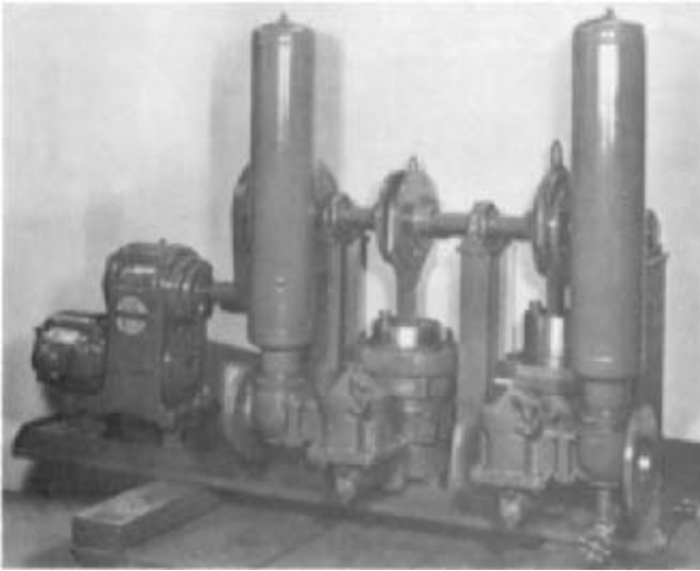
FIGURE 9 Plunger-type sludge pump (ITT Marlow Pumps)
