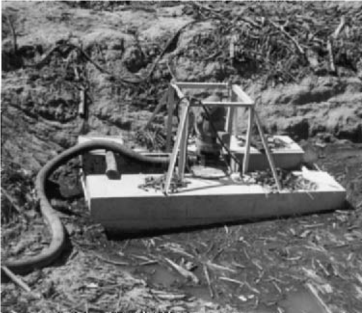
FIGURE 1 A simple barge (Hazleton Pumps, Inc.)
