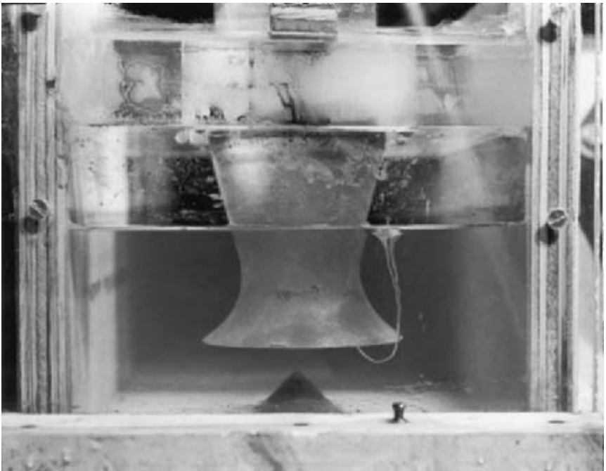
FIGURE 1B Free surface vortex can form at pump suction bell entrance due to combination of low submergence, high suction velocity, nonuniform approach flow, or other vorticity sources (Courtesy of Alden Research Laboratory, Inc.)
